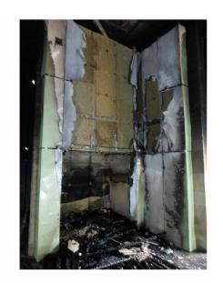
Figure 3 - Stone wool insulated system with A2 ACM panels
