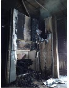
Figure 4 - PIR insulated system with A2 ACM panels
