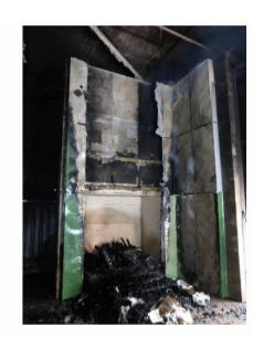
Figure 5 - Phenolic insulated system with A2 ACM panels
