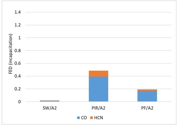
Figure 17 – Contribution of CO and HCN to incapacitation at 30 minutes for gases entering a 50m³ room from cladding through 100mm vent
