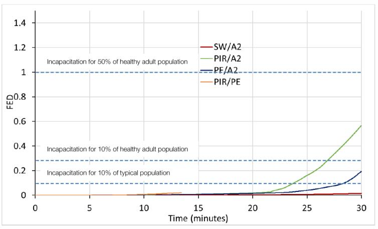
Figure 16 – Total FED for incapacitation for gases entering a 50m³ room from cladding through 100mm vent (The curve for PIR/PE is shown until the wood crib was extinguished at 12 minutes)
