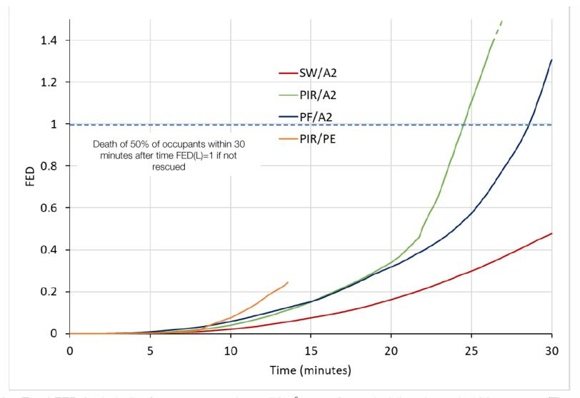
Figure 18 – Total FED for lethality for gases entering a 50m³ room from cladding through 100mm vent (The curve for PIR/PE is shown until the wood crib was extinguished at 12 minutes)
